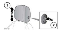
1. To raise, pull the head restraint upwards. It will click and lock in to position.
