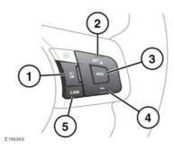
The Cruise control system is operated by controls mounted on the steering wheel. The driver can also intervene at any time, by use of the brake or accelerator pedals.
