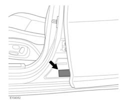
The recommended tyre pressures are listed on a label, located on the driver's side B pillar. Open the driver's door to access the tyre pressure label.
