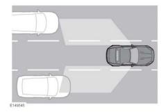
The Blind Spot Monitor (BSM) system monitors a zone that covers the area adjacent to the vehicle, that is not easily visible by the driver and is designed to help identify any object passing the vehicle.
