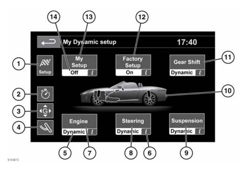
Vehicles with configurable dynamics, allow the Dynamic mode settings to be configured via the Touch screen for selected characteristics, with a choice between Normal and Dynamic settings. See **69**, **EXTRA FEATURES**.
