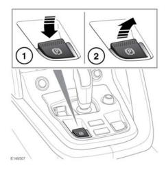
With the ignition switched on, press the brake pedal and press down on the EPB switch (1). This will release the Parking brake.
