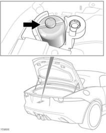
The tire repair kit consists of a canister of sealant located below the Luggage compartment left-side (battery) cover, in front of the vehicle's battery, as shown, and a compressor located in the Luggage compartment.
