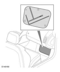
Remove the 2 tools from behind the passenger footwell fuse box cover. See **176**, **FUSE BOX LOCATIONS**.
