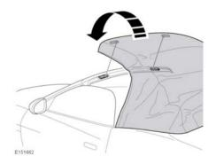
Carefully raise the roof to the closed position. An increase in effort is required to reach the fully closed position.
