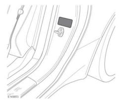
A tire information label is located in the driver's door opening, giving information specific to the original wheel and tire equipment fitted to the vehicle.
