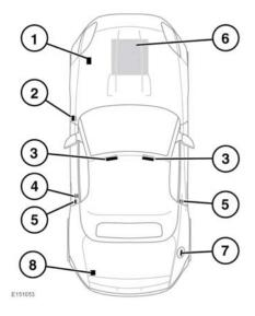
Air conditioning label - Left side inner fender. 2. Vehicle identification plate, including the Vehicle Identification Number (VIN) and recommended maximum vehicle weights - Left side B pillar.
