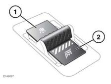
**Note:** Automatic transmission: The switch lever will always return to the center position when released, regardless of the mode selection.
