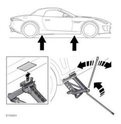
There are 4 jacking points on the underside of the floor. Two indented, triangular indicators are provided on each sill cover. These indicate the location for the jack.
