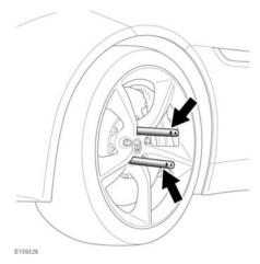
On vehicles with carbon ceramic brake rotors, remove 2 opposing wheel nuts and install the 2 wheel guide pins, as shown.
