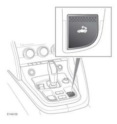
The power-operated convertible roof is controlled by a switch located on the center console, as illustrated. The ignition system must be on. The roof will latch and unlatch automatically. The roof can be operated at speeds below 30 mph (50 km/h). However, for safety it should not be opened or closed when the vehicle is being driven.
