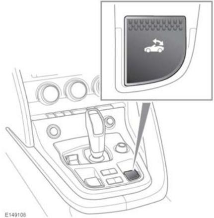
The power-operated convertible roof is controlled by a switch located on the center console, as illustrated. The ignition system must be on. The roof will latch and unlatch automatically. The roof can be operated at speeds below 30 mph (50 km/h). However, for safety it should not be opened or closed when the vehicle is being driven.
