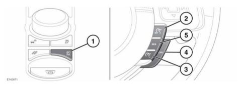
ASL allows a speed limit to be set that the driver does not wish to exceed.
