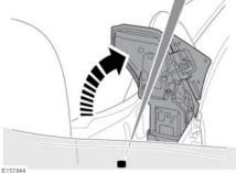
Lift the panel. With the allen key, unscrew and remove the bolt.
