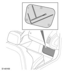
Remove the 2 tools from behind the passenger footwell fuse box cover. See **163**, **FUSE BOX LOCATIONS**.
