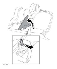
Lift the panel. A gradual increase of effort is required to reach the illustrated vertical position. Using the flat blade of the allen key tool, lightly pry off the control rod ball socket.
