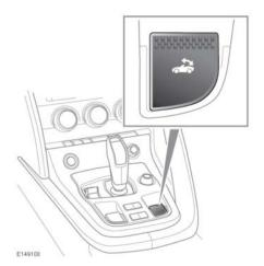
The power-operated convertible roof is controlled by a switch located on the centre console, as illustrated. The ignition system must be on. The roof will latch and unlatch automatically. The roof can be operated at speeds below 50 km/h (30 mph). However, for safety it should not be opened or closed when the vehicle is being driven.
