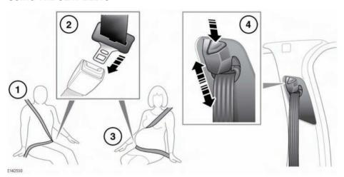
Putting on a seat belt: Draw the belt out smoothly, make sure that the belt height, the seat and the occupant's position on the seat, are correct.
