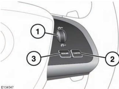
The system is operated by controls mounted on the steering wheel. The driver can also intervene at any time by use of the brake or accelerator pedals.
