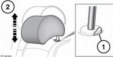
1. If the head restraint is to be lowered, press and hold the locking collar, and then push the head restraint down to the required position.
