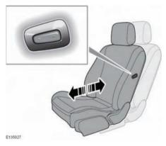
This feature allows the fore and aft position of the front passenger seat to be adjusted from the driver seat and rear passenger seats. Press the front of the button to move the seat forwards. Press the rear of the button to move the seat rearwards.
