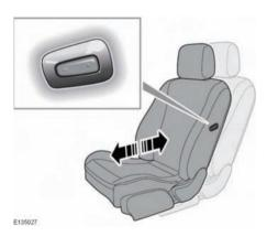
This feature allows the fore and aft position of the front passenger seat to be adjusted from the driver seat and rear passenger seats. Press the front of the button to move the seat forwards. Press the rear of the button to move the seat rearwards.
