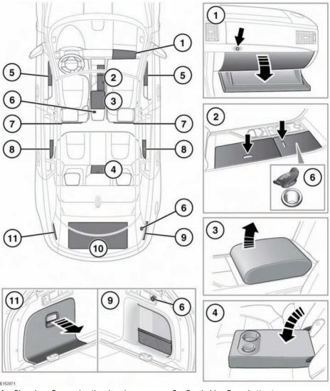
1. Glove box: Open using the glove box release (arrowed).
