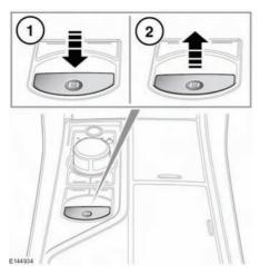
With the ignition turned on, press the brake pedal and press down on the EPB switch (1). This will release the electronic parking brake.
