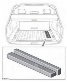
For Sportbrake models, a warning triangle is stored in a rear floor recess.
