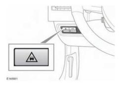
Press the button to switch Forward alert on or off.
