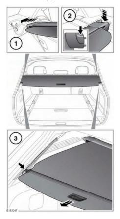
With the tailgate open and the rear seats folded forward, engage the left end of the assembly into the moulded recess in the left side of the loadspace.
