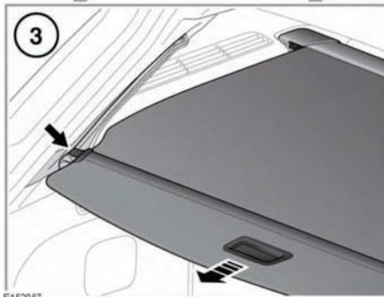
1. With the tailgate open and the rear seats folded forward, engage the left end of the assembly into the moulded recess in the left side of the loadspace.
