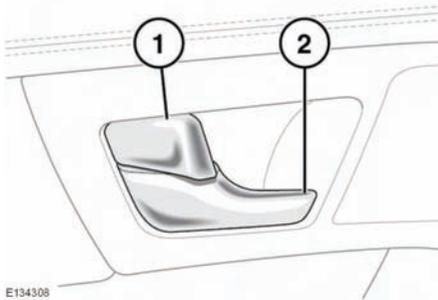
1. Press the locking lever to lock the door. Pull the lever to unlock the door. Operating the locking lever on either front door will lock or unlock all closed doors.
