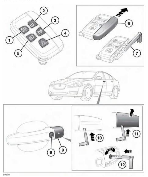
1. Press the lock button to secure the vehicle. The vehicle can be Single or Double locked.
