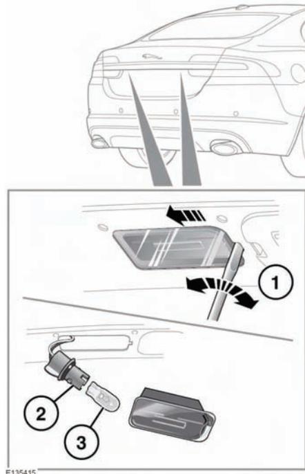
1. Insert a small flat-bladed screwdriver into the indent as shown and carefully lever out the side of the lamp unit and remove.
