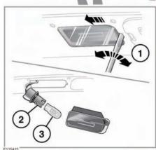
Insert a small flat-bladed screwdriver into the indent as shown and carefully lever out the side of the lamp unit and remove.
