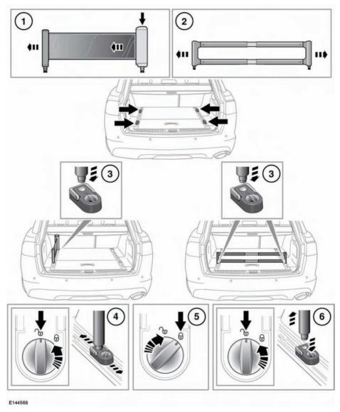
For Sportbrake models, a luggage divider kit is provided to assist with safely securing items of
