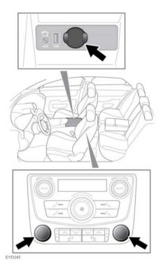
To access the auxiliary power sockets, remove or pull out the protective cover.
