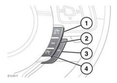
SET+: Press to set the speed or to increase the set speed. The cruise control warning lamp will illuminate to confirm cruise control is operational (see 42, CRUISE CONTROL (GREEN)).
