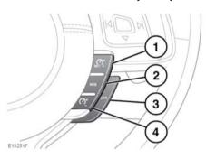
SET+: Press to set the speed or to increase the set speed. The cruise control warning lamp will illuminate to confirm cruise control is operational (see 42, CRUISE CONTROL (GREEN)).
