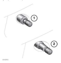
Wheels fitted with TPMS can be visually identified by the external metal lock nut and valve (1). All Jaguar non-TPMS wheels have a rubber valve fitted (2).
