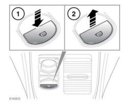
The switch which operates the parking brake is mounted on the centre console to the rear of the gear selector.
