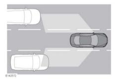
The Blind Spot Monitor (BSM) system monitors a zone that covers the area adjacent to the vehicle, that is not easily visible by the driver and is designed to identify any object overtaking the vehicle. The system uses a radar on each side of the vehicle to identify any overtaking vehicle/object within the blind spot area of the vehicle, while disregarding other objects which may be stationary or travelling in the opposite direction, etc.
