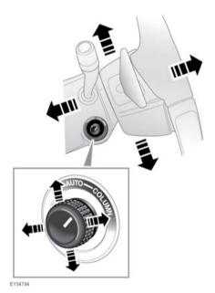
The steering wheel can be adjusted for tilt and reach as follows:
