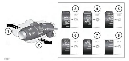
With the headlamps on, push the switch away from the steering wheel to select high beam. The blue warning indicator on the instrument panel will illuminate.
