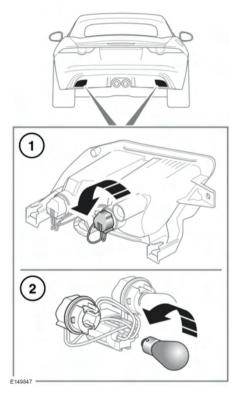
Access to the 3.0L vehicle's reverse lamp housing is from underneath the rear bumper.
