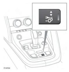
Press the switch to manually deploy the DRS at speeds below 96 km/h (60 mph). The switch will illuminate to confirm.
