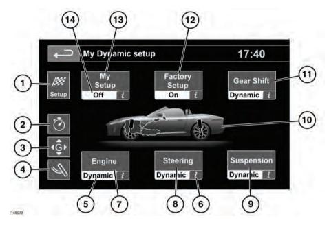
Vehicles with configurable dynamics, allow the dynamic mode settings to be configured via the touch screen for selected characteristics, with a choice between Normal and Dynamic settings. Touch Extra features on the Home menu screen. See 53, TOUCH SCREEN HOME MENU.
