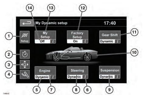
Vehicles with configurable dynamics, allow the dynamic mode settings to be configured via the touch screen for selected characteristics, with a choice between Normal and Dynamic settings. Touch **Extra features** on the **Home menu** screen. See **53**, **TOUCH SCREEN HOME MENU**.
