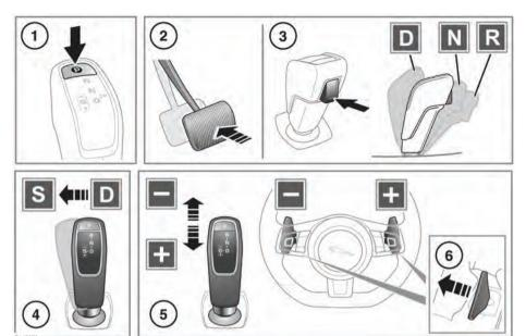
Gear selector status is displayed in the Message centre. See **31, INSTRUMENT PANEL**. Also the appropriate LED indicator, on top of the gear selector, will illuminate to confirm selection.
