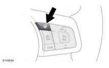
To activate the heated steering wheel, press the switch. Press again to turn off.
