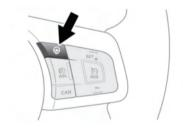
To activate the heated steering wheel, press the switch. Press again to turn off.
