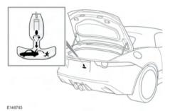
The release handle glows in the dark and is located inside the luggage compartment as illustrated. To open the luggage compartment from the inside, pull the handle while pushing the luggage compartment lid upwards.
