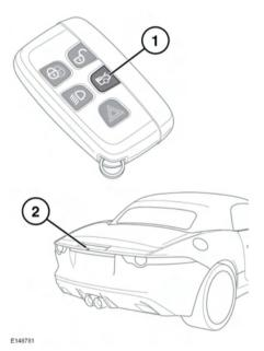
The luggage compartment can be opened using the appropriate button on the Smart Key (1), or via keyless entry, see 8, KEYLESS ENTRY. It can also be opened using the exterior release (2), provided the doors are unlocked and Park (P) is engaged.
