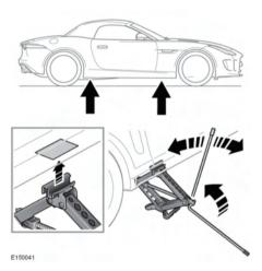
There are four jacking points on the underside of the floor. Two indented, triangular indicators are provided on each sill cover. These indicate the location for the jack.
