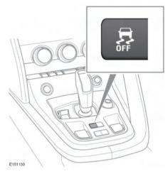
Press and hold the DSC switch for more than 3 seconds.
