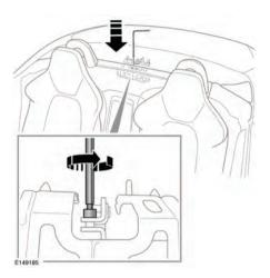
Using the allen key tool, rotate the release screw 7 turns counter clockwise to release the down-lock mechanism.
