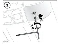
Remove the access plug from the centre of the roof header trim. Insert the screw thread end of the tool into the motor shaft. To fully engage, rotate clockwise until resistance is felt. It does not need to be tight. 2. Pull the tool to remove the motor shaft.
