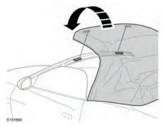
Carefully raise the roof to the closed position. An increase in effort is required to reach the fully closed position.
