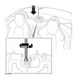
Using the allen key tool, rotate the release screw 7 turns counter clockwise to release the down-lock mechanism.
