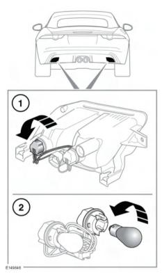
Access to the 3.0L vehicle's rear fog lamp housing is from underneath the rear bumper.
