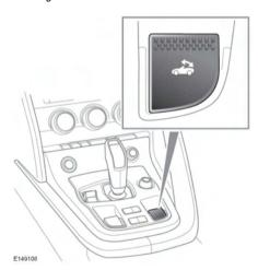
The power operated convertible roof is controlled by a switch located on the centre console. The ignition system must be on. The roof will latch and unlatch automatically. The
